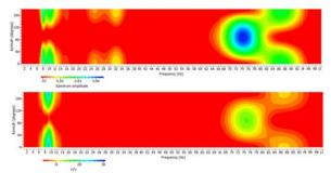
Figure 4: Directional plots: A) Density Spectrum; B) H/V ratio
