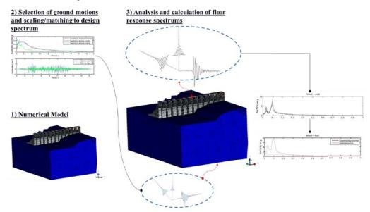
Figure 9: Methodology to calculate floor response spectrum
