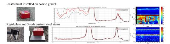
Figure 7: Effect of a rigid plate on measures: A) Without rigid plate; B) With the rigid plate
