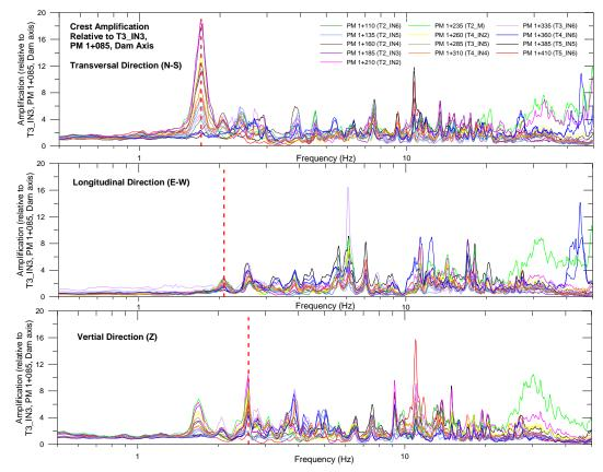
Figure 12: Transfer functions calculated from ambient noise measurements of top of the Denis-Perron dam
